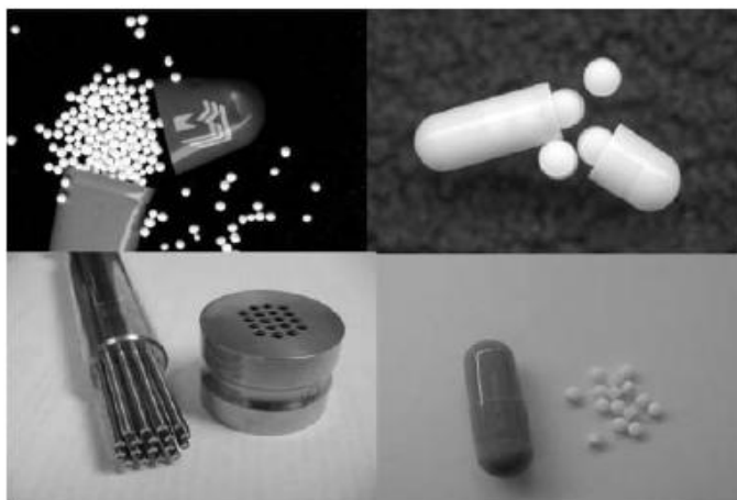
FIGURE 21.2 Examples of beads and mini-tablets prepared with single-head or multi-head tooling
