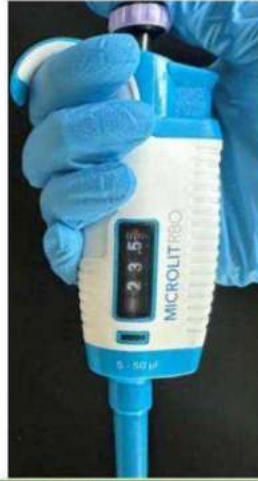
P-50, range (5-50 \mu L) Display: 23.5 \mu L
