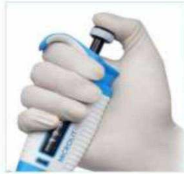
Position 2 (First Stop) is reached by pushing down on the plunger until resistance is met
