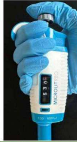
P-1000, range (100-1000 \mu L) Display: 530 \mu L
