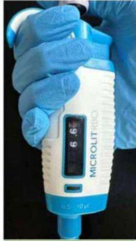
P-10, range (0.5-10 \mu L) Display: 6.6 \mu L
