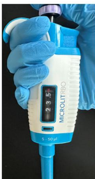
P-50, range (5-50 \mu L) Display: 23.5 \mu L
