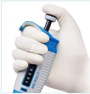
Position 1 is where the pipette is at rest
