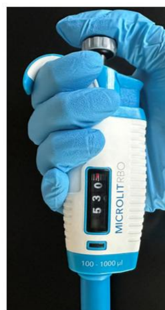
P-1000, range (100-1000 \mu L) Display: 530 \mu L
