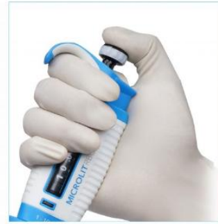
Position 3 (Second Stop) is reached by pushing down from position 2
