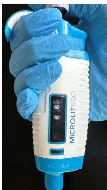
P-10, range (0.5-10 \mu L) Display: 6.6 \mu L
