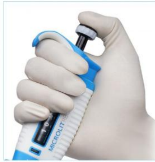
Position 2 (First Stop) is reached by pushing down on the plunger until resistance is met
