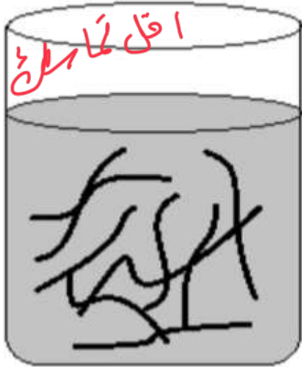
Figure 1. Gel formation due to swelling of gelling agent
